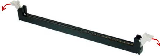
3. Align the memory module on the socket making sure that the notch matches the break on the socket.
