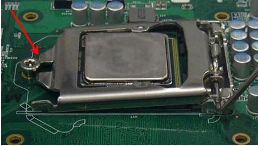
8. Lower the locking arm and fasten it to the retention tab (A). The load plate should be locked underneath the screw as shown (B).
